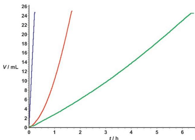
Figure 3. Comparison of hydrogen consumption curves of the hydrogenation of methyl (*Z*)- $\alpha$ -acetamido cinnamate (MAC) with different dipamp complexes:  $[\text{Rh}(\text{dipamp})(\text{MeOH})_2]\text{BF}_4$  (blue),  $[\text{Rh}(\text{dipamp})(\text{cod})]\text{BF}_4$  (red),  $[\text{Rh}_3(\text{dipamp})_3(\mu_3\text{-OH})_2]\text{BF}_4$  (green); each 0.01 mmol Rh; 1.0 mmol MAC; 15.0 mL methanol; 25.0 °C; 101.3 kPa.<sup>[18]</sup>
