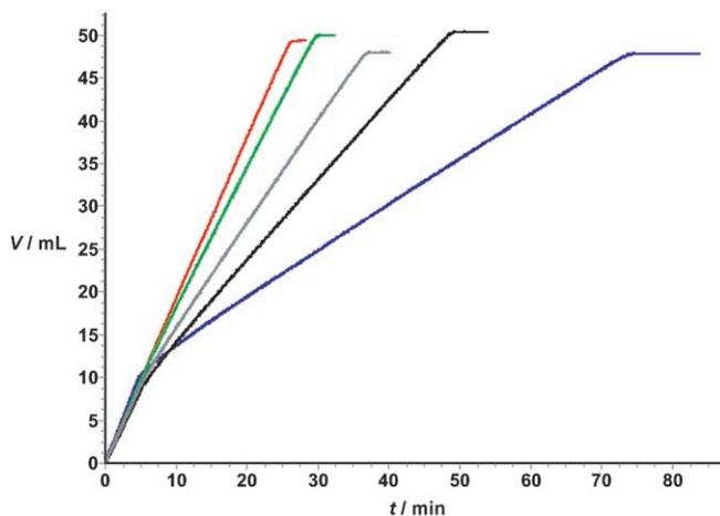
Figure 4. Hydrogen consumption curves of the hydrogenation of MAC with  $[\text{Rh}(\text{dipamp})(\text{MeOH})_2]\text{BF}_4$  (red). Addition of  $\text{NEt}_3$  to analogous hydrogenations after ca. 20% conversion: green = 0.01 mmol, gray = 0.05 mmol, black = 0.1 mmol, blue = 0.35 mmol (each 0.01 mmol Rh; 2.0 mmol MAC; 15.0 mL methanol; 25.0 °C; 101.3 kPa).
