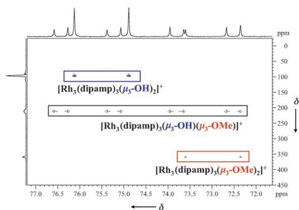
Figure 2.  $^{31}\text{P}$ - $^{103}\text{Rh}$  HMQC spectrum of trinuclear Me-DuPhos complexes with different  $\mu_3$ -bridging anions in  $\text{CD}_2\text{Cl}_2$ .<sup>[14]</sup>
